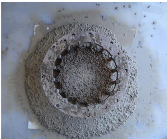
**Figure 5.7: J-Ring Flow Spread of Mixture # 25**
