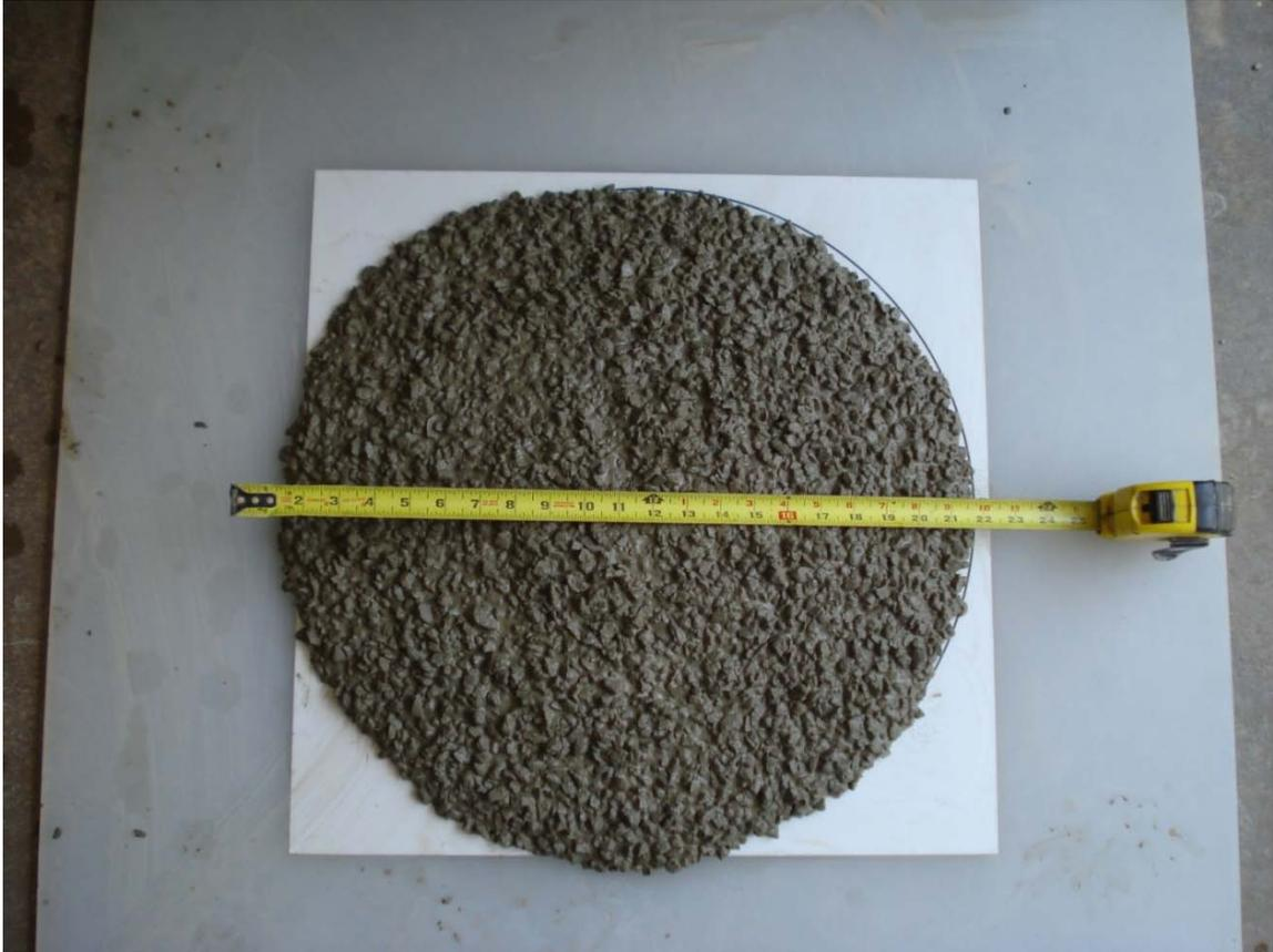
**Figure 5.5: Slump Flow of Mixture # 15**
