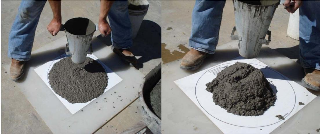
**Figure 6.13: Evidence of the Declining Effectiveness of HRWR at an Extended Batching Time**
