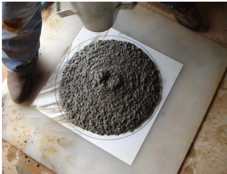
**Figure 5.16: Slump Flow of Mixture # 49**
