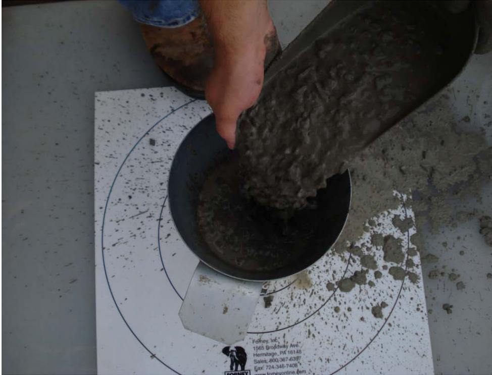
**Figure 3.6: Filling the Slump Cone**
