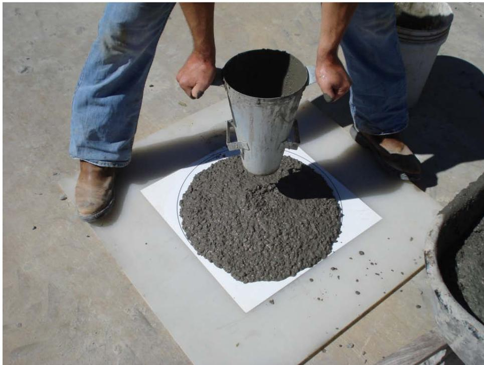
**Figure 3.7: Lifting the Slump Cone**
