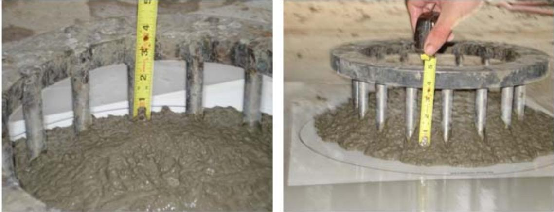
**Figure 3.14: Measuring SCC Height Difference**
