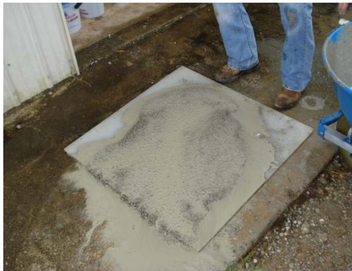
**Figure 3.12: Mixture with VSI equal to 3**
