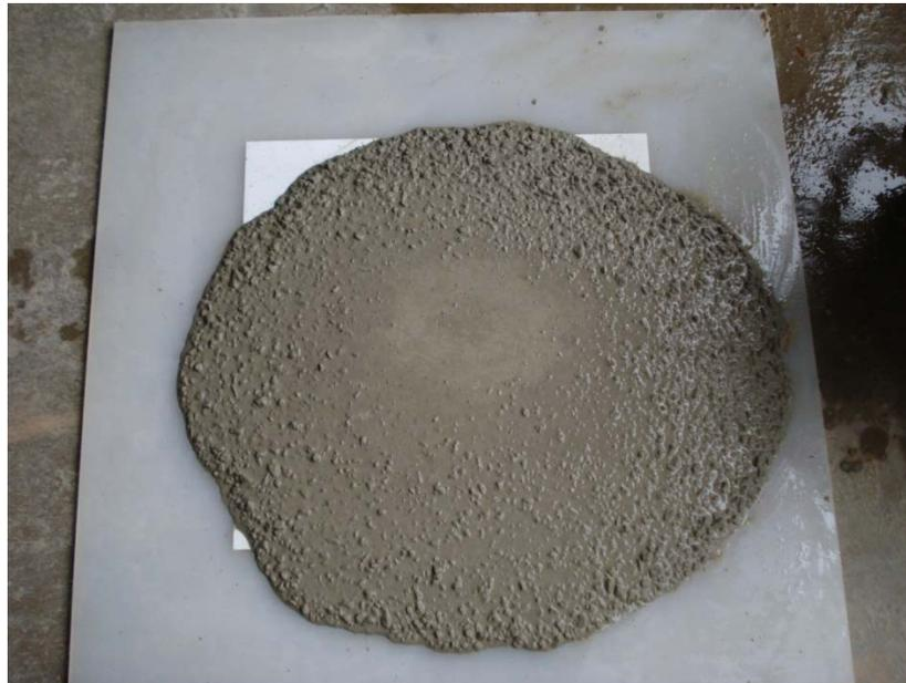
**Figure 5.3: Slump Flow of Mixture # 7**
