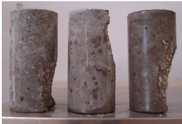
**Figure 3.16: SCC Cylinders Tested in Compression**
