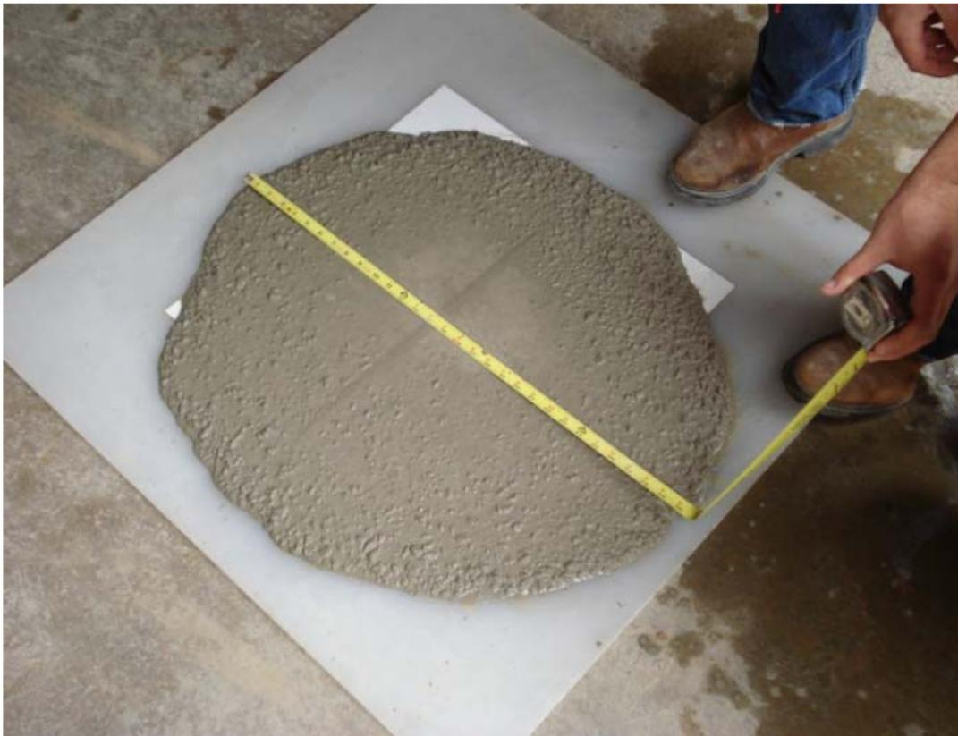
**Figure 3.10: Mixture with VSI equal to 1**
