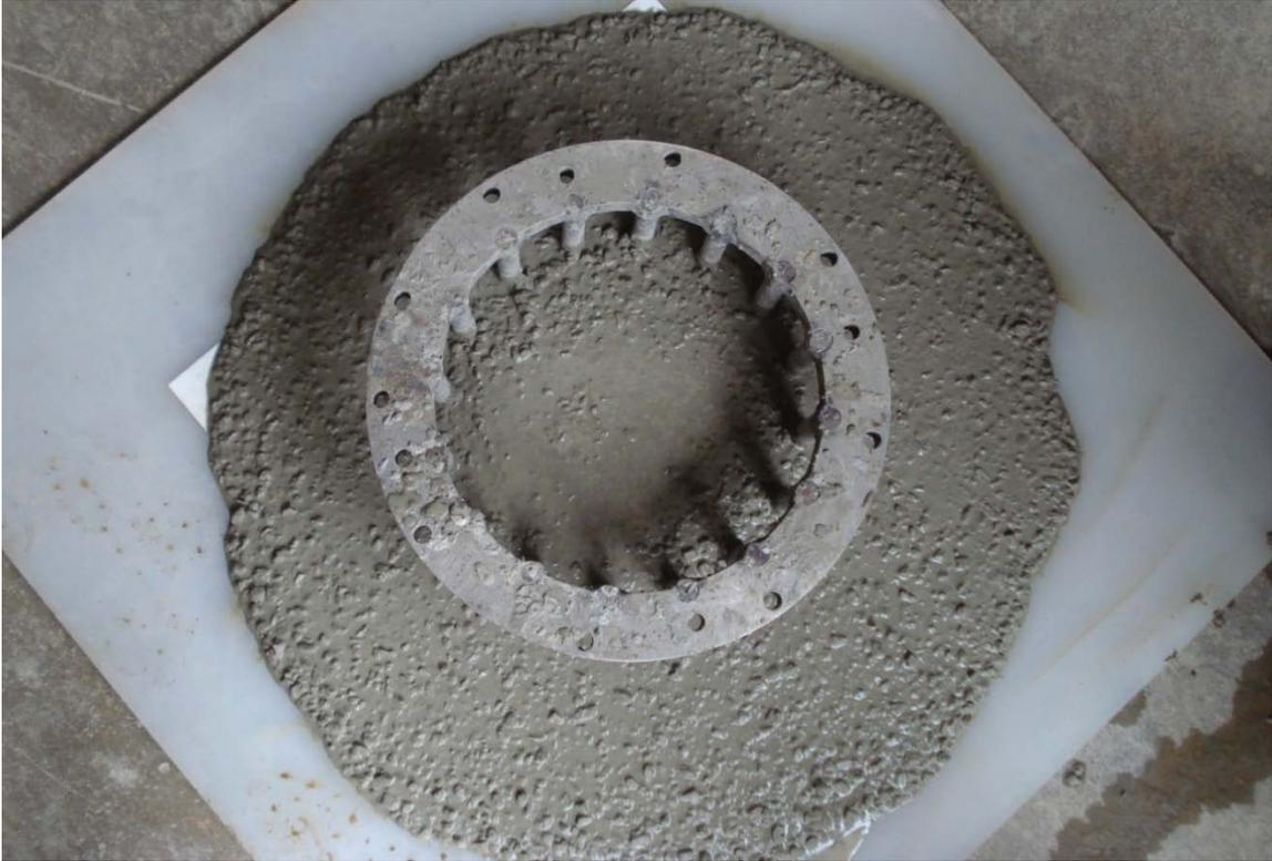
**Figure 2.6: View of J-Ring Flow Spread**
