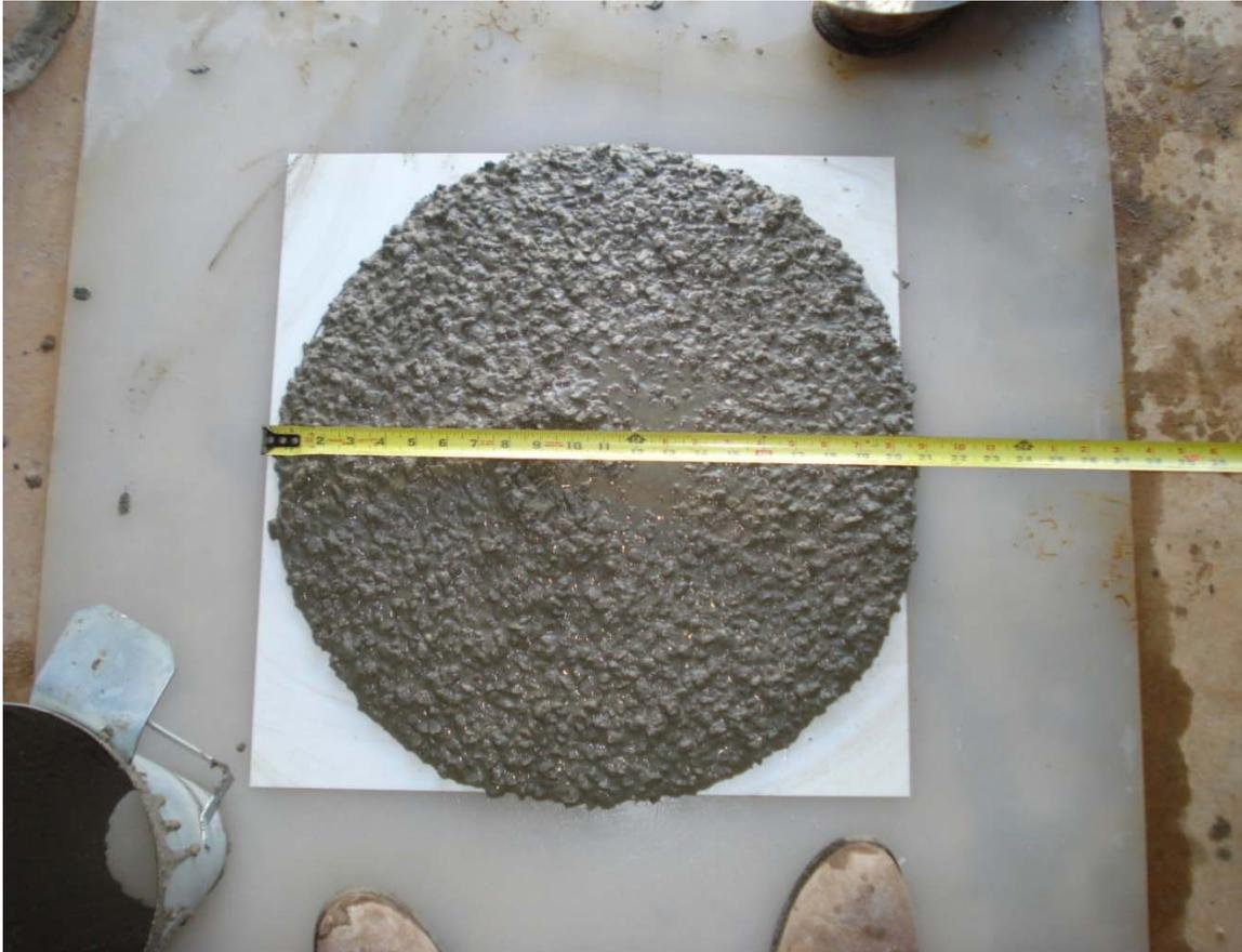
**Figure 2.4: View of Slump Flow Spread**
