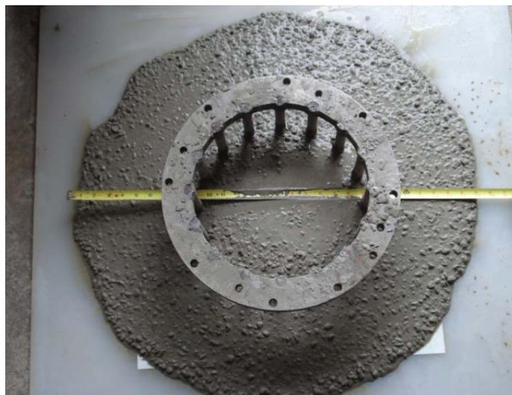
**Figure 3.15: Measuring the J-Ring Flow Spread**
