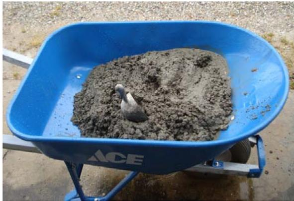
**Figure 6.8: Sample of Trial Batch # 1a Before HRWR was Added**
