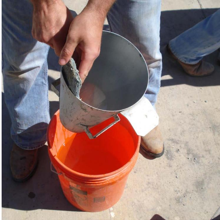
**Figure 3.5: Wetting the Slump Cone**
