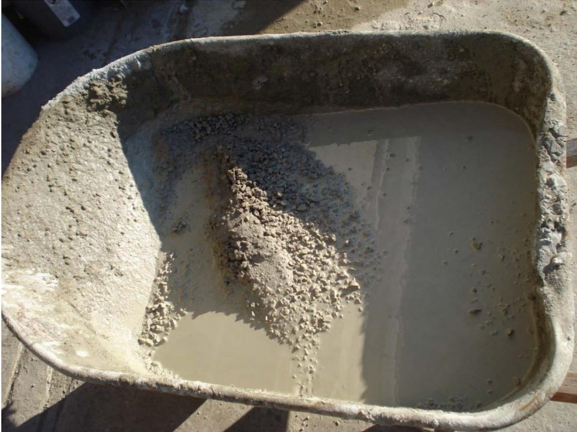
**Figure 5.11: Evidence of Segregation in Mixture # 36**
