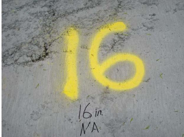
Figure 4.2: Wall 16 Showing Poor Slump Flow
