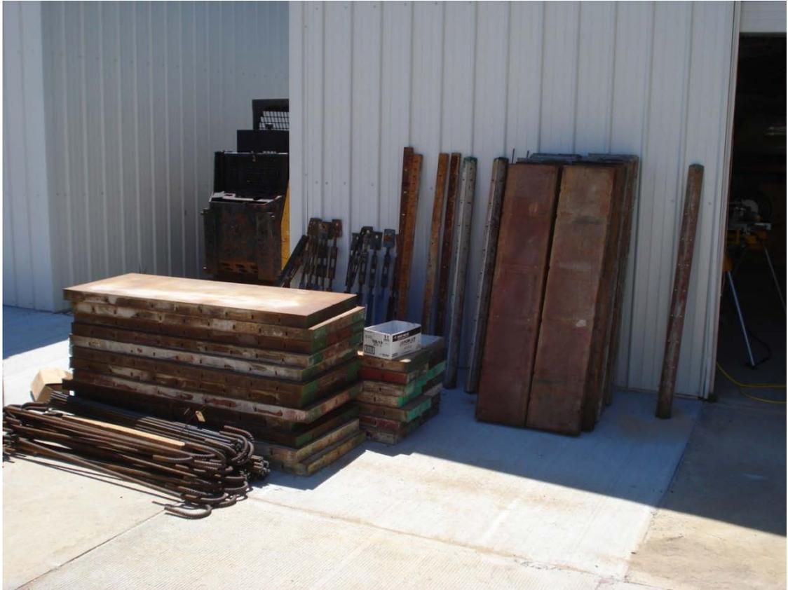
**Figure 6.2: Steel-ply Formwork and Rebar**
