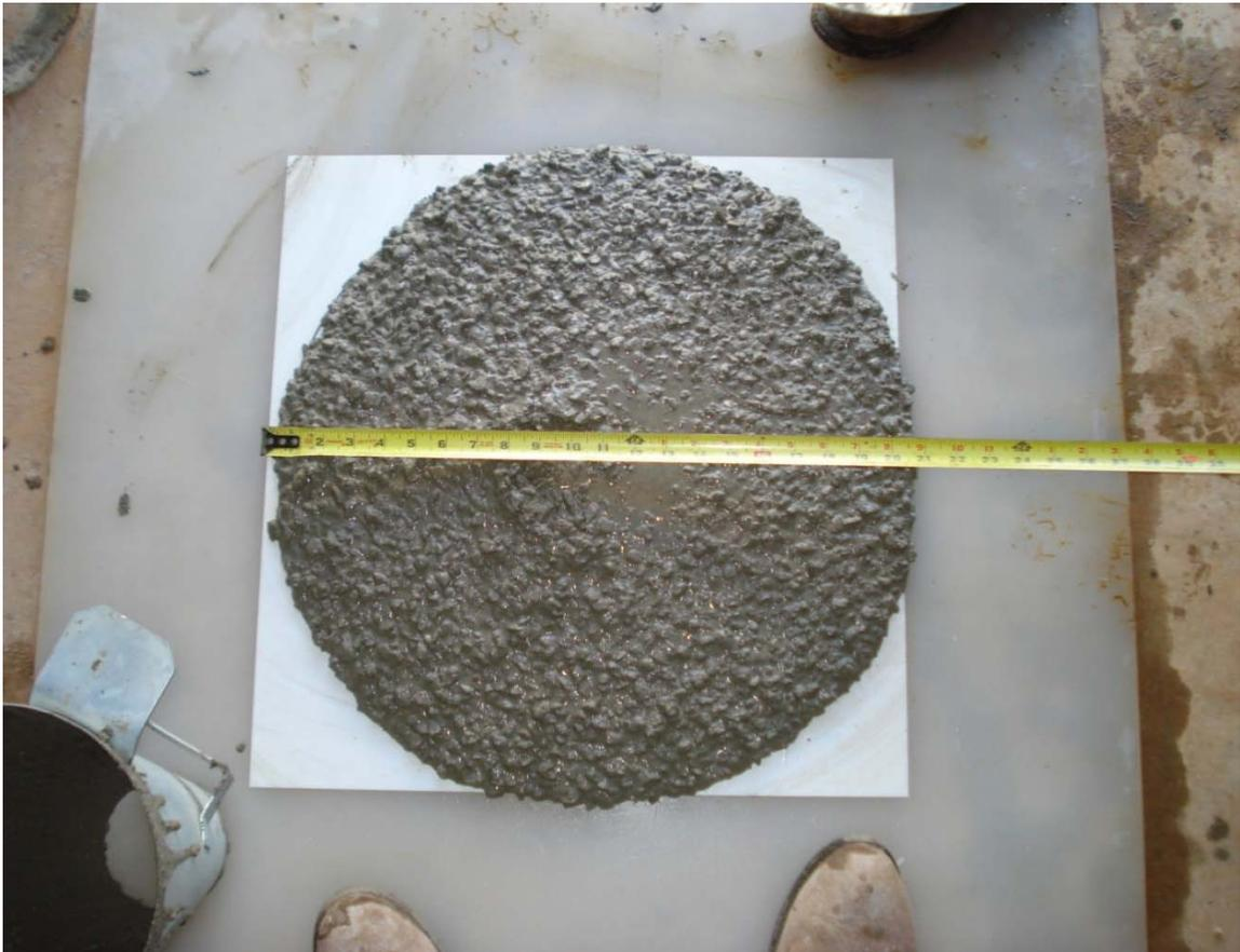
**Figure 2.4: View of Slump Flow Spread**
