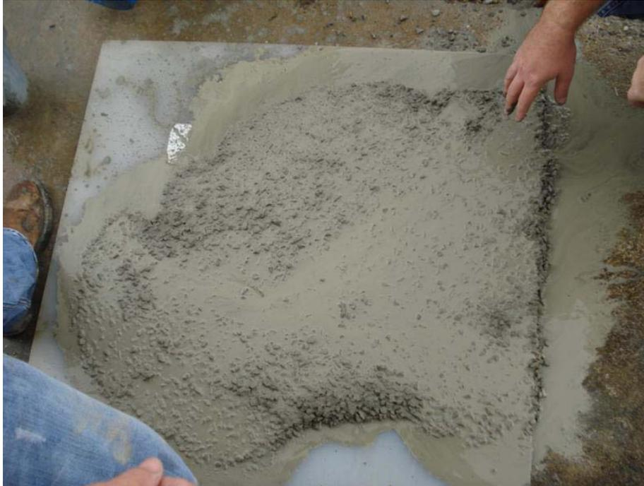
**Figure 6.12: View of Slump Flow Spread for Trial Batch # 1a**
