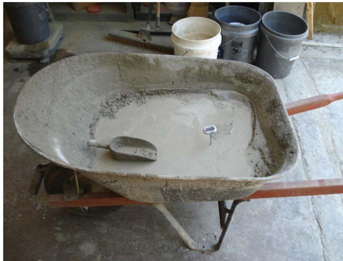
**Figure 5.15: Instability Observed in Mixture # 44**
