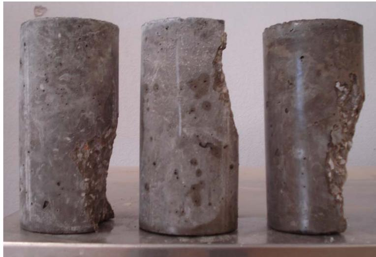
**Figure 3.16: SCC Cylinders Tested in Compression**
