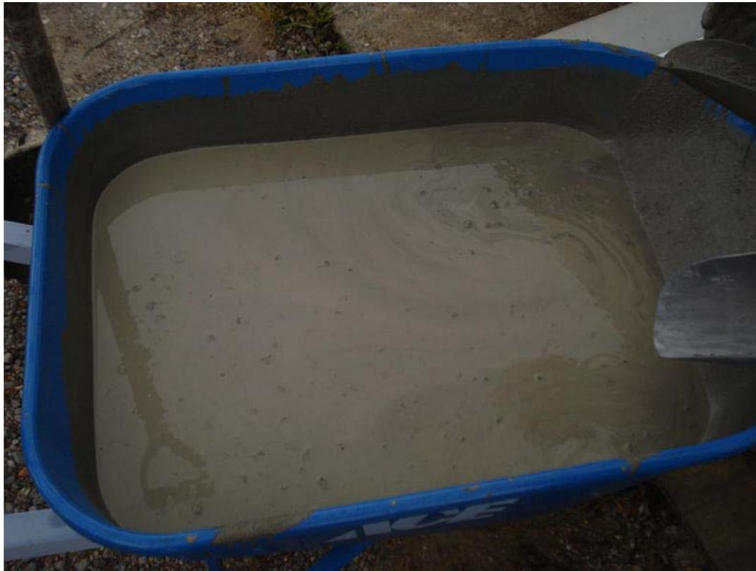
**Figure 6.11: Segregation Observed in Trial Batch # 1a**
