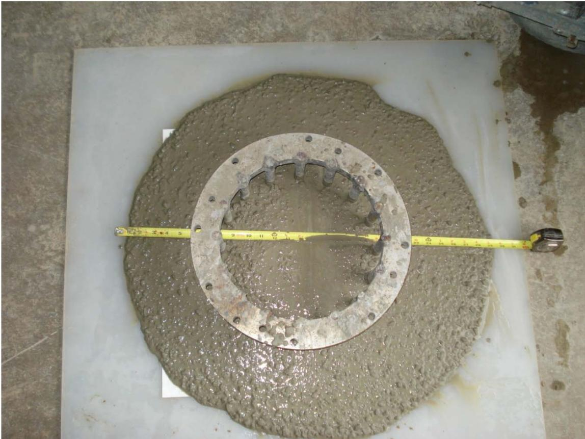
**Figure 5.6: J-Ring Flow Spread of Mixture # 20**
