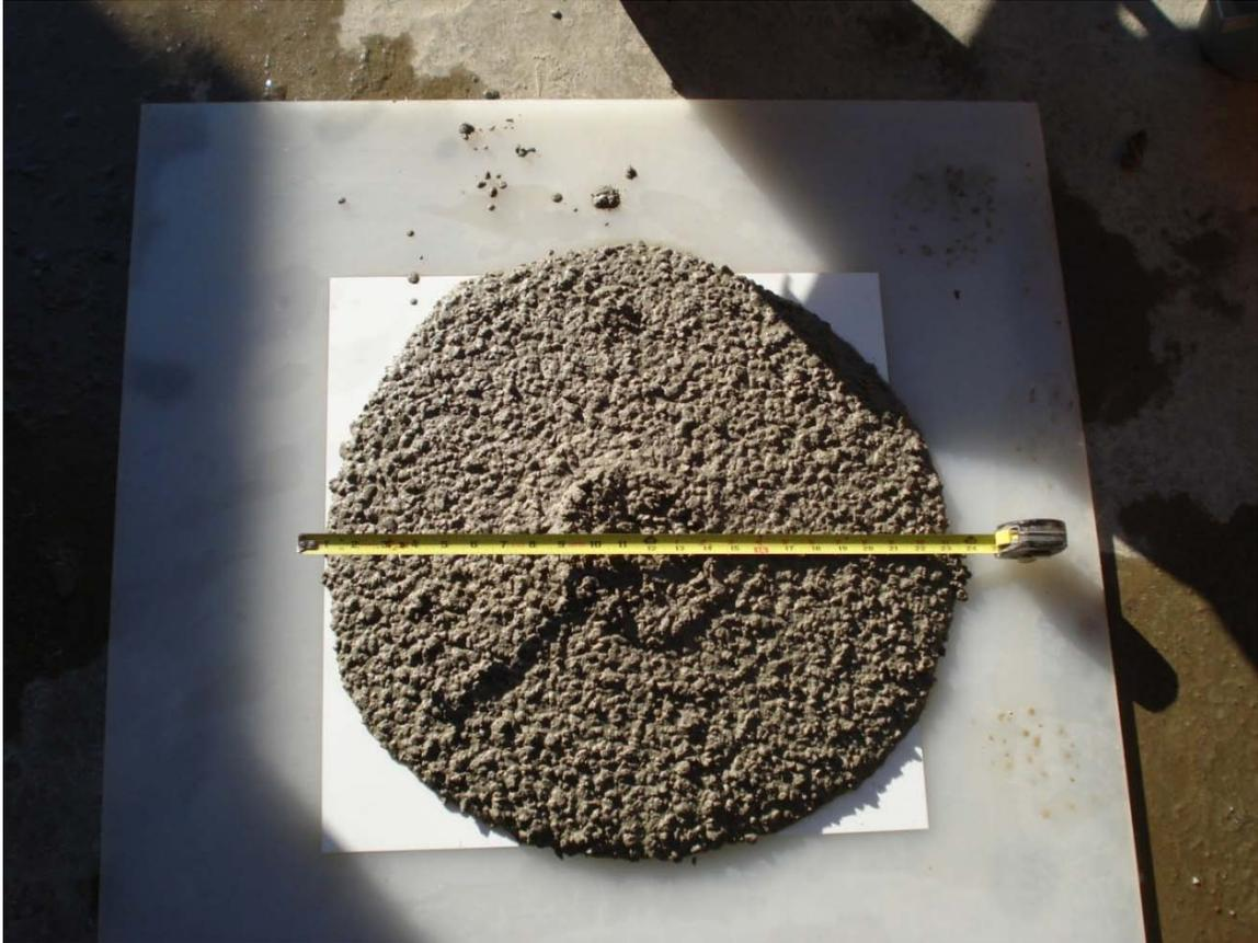
**Figure 5.17: Slump Flow of the Final Mixture**
