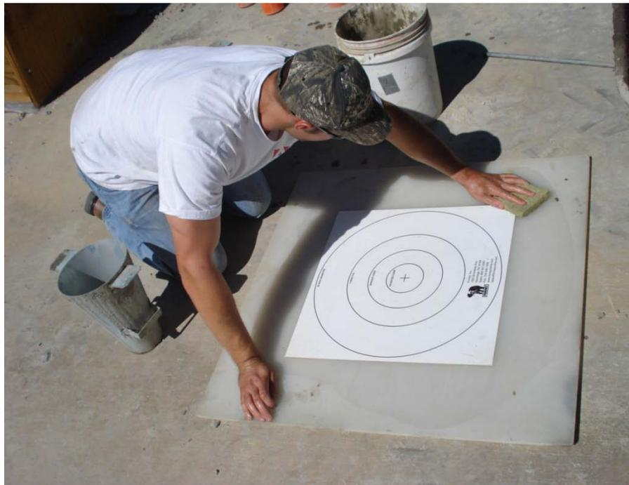
**Figure 3.4: Dampening the Slump Flow Board**
