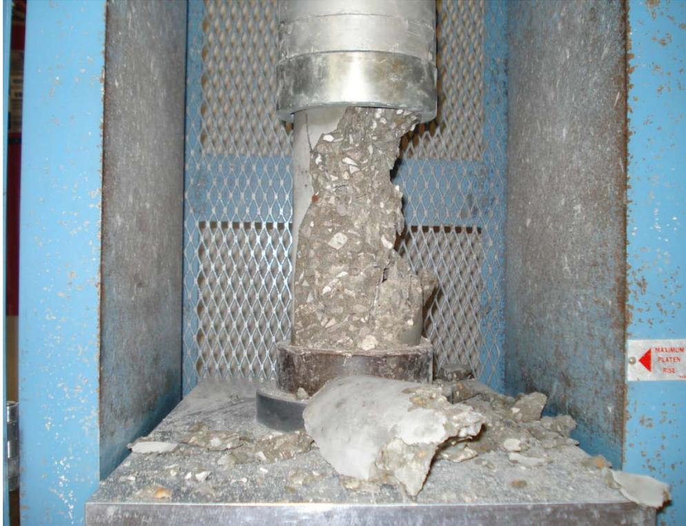
**Figure 5.8: 28-Day Compressive Strength Testing on Cylinder Cast from Mixture # 29**
