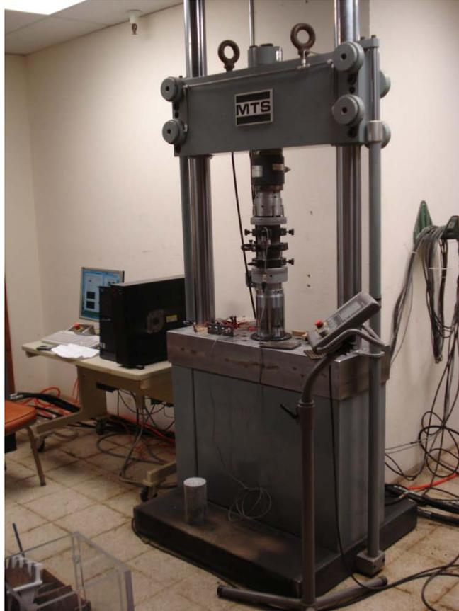
**Figure 3.17: DAQ and Apparatus used for Modulus of Elasticity Testing**
