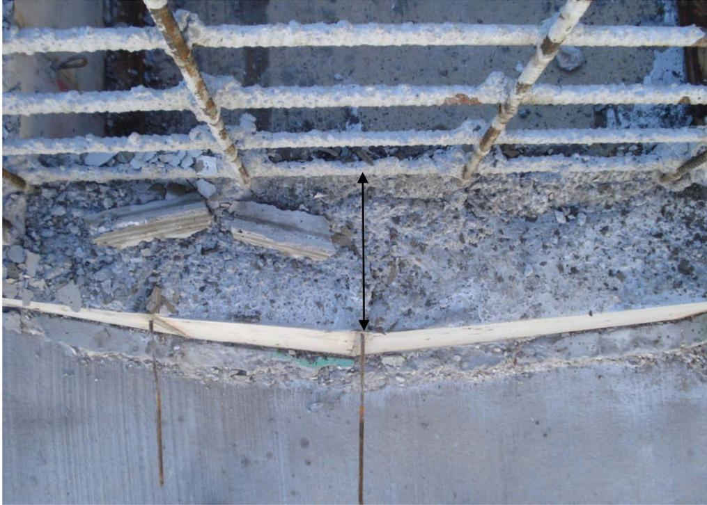
**Figure 6.15: Critical Location Where Failure Occurred in Box Culvert # 1**
