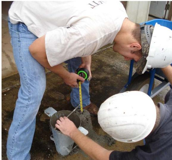
**Figure 6.9: Conducting Slump Test on Sample of Trial Batch # 1a**
