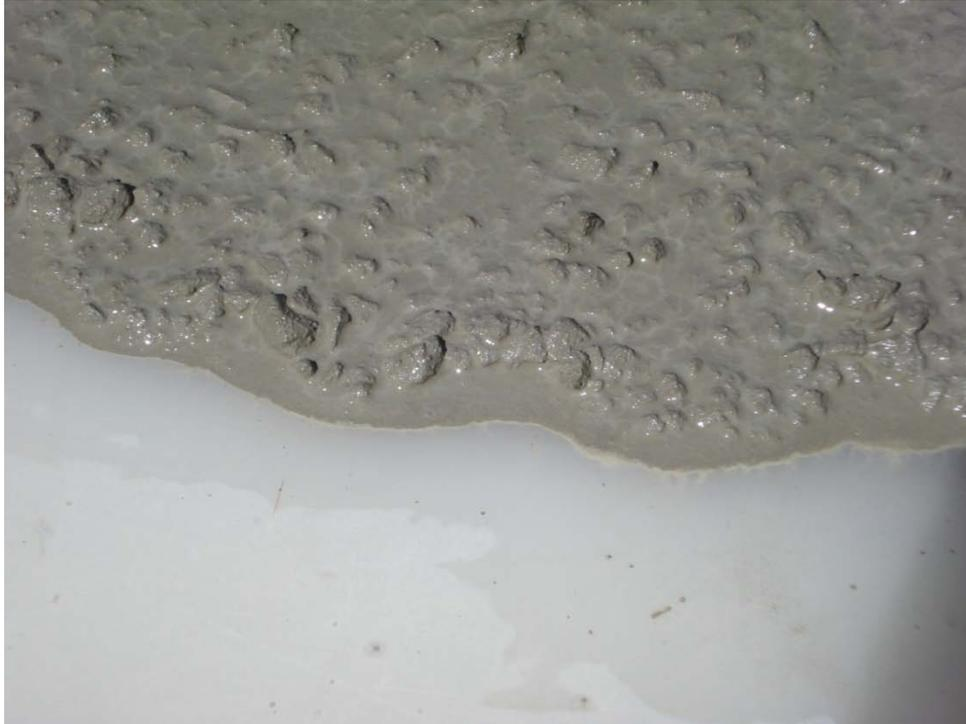
**Figure 6.23: Bleed Water Observed in Mixture Used for Casting Box Culvert # 2**
