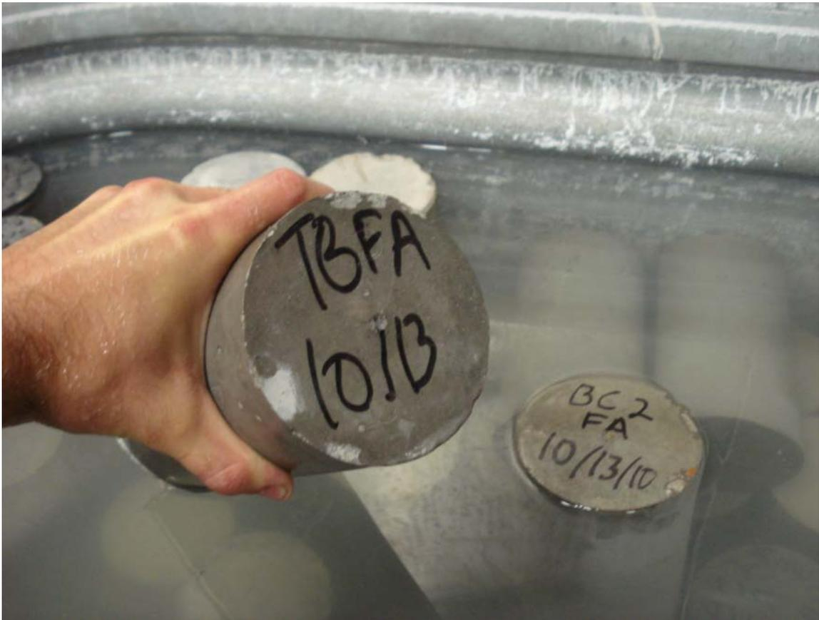
**Figure 3.18: Labeled Cylinders Curing in Lime Saturated Water**
