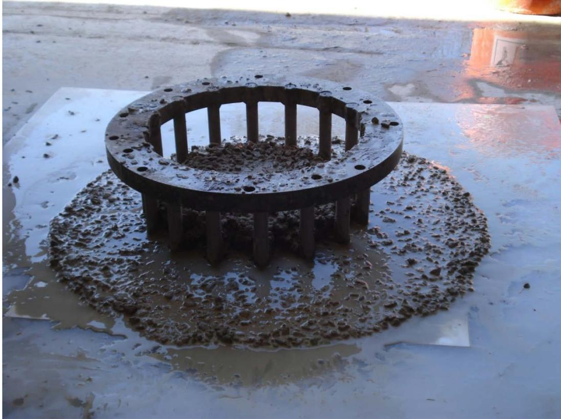
**Figure 5.12: J-Ring Flow Spread of Mixture # 38**
