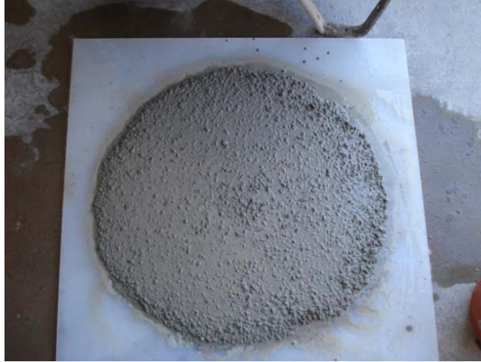
**Figure 3.11: Mixture with VSI equal to 2**
