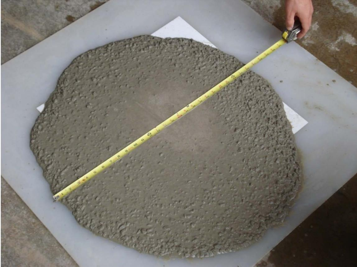
**Figure 3.8: Measuring the Slump Flow Spread**
