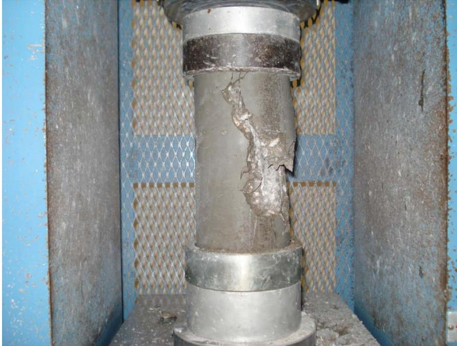
**Figure 5.14: Shear-Type Compression Failure**
