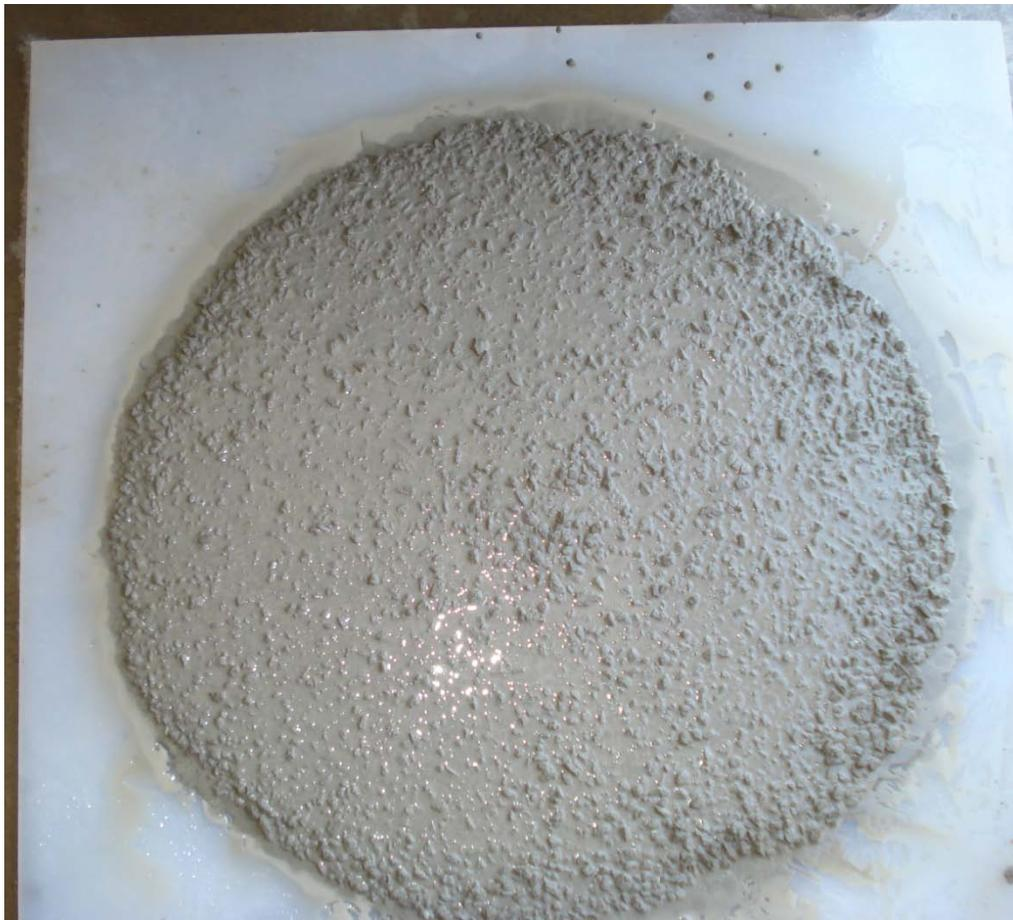
**Figure 5.13: Slump Flow of Mixture # 39**
