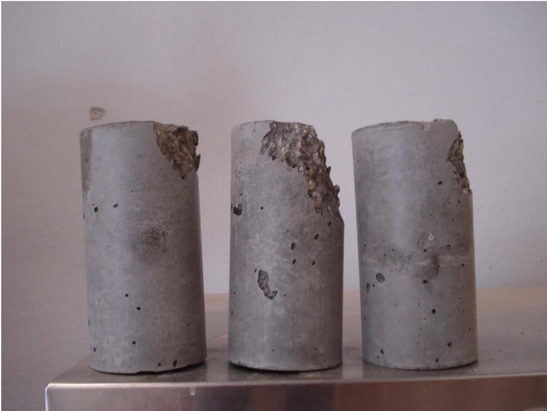
**Figure 5.10: Compressive Strength Cylinders for Mixture # 34 at 28 Days**
