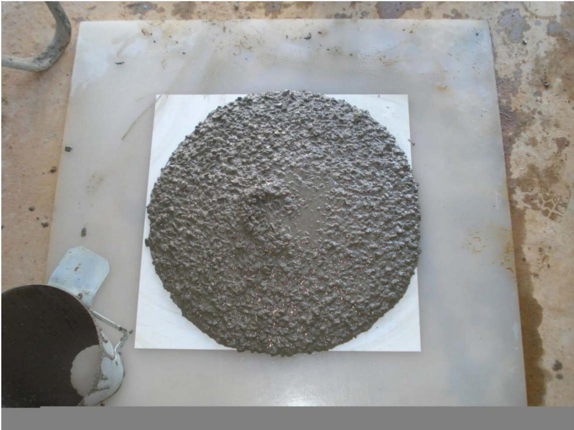
**Figure 2.5: Approximate Concrete Spread Diameter at which the T-20 (T-50) Test Ends**
