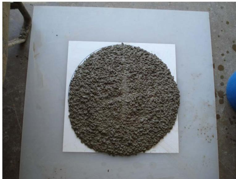
**Figure 5.9: Slump Flow of Mixture # 31**
