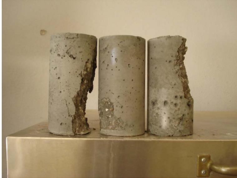
**Figure 5.4: Compressive Strength Cylinders for Mixture # 12 at 28 Days**
